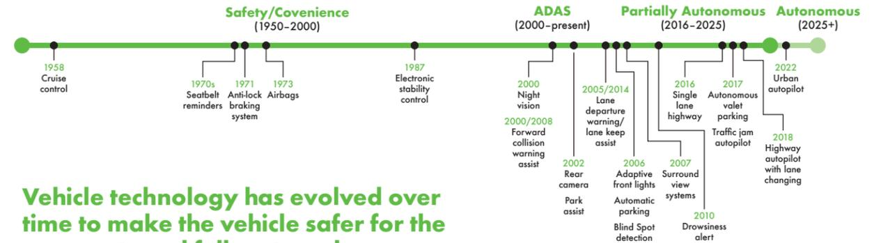
**Vehicle technology has evolved over time to make the vehicle safer for the occupants and fellow travelers.**
