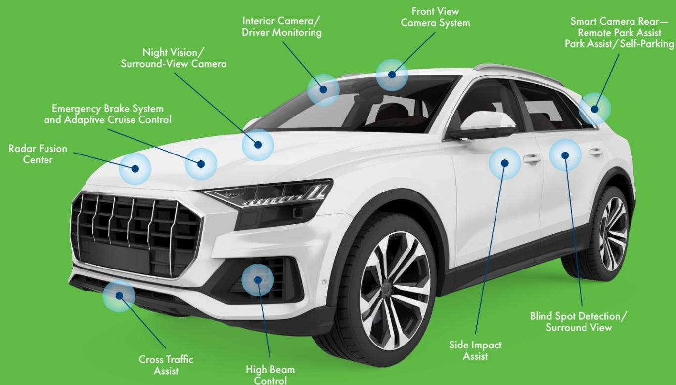
Right now, close to 60 million vehicles in the U.S. are equipped with some sort of ADAS (advanced driver-assistance systems) technology, like parking assistance, adaptive cruise control, or collision avoidance systems. By 2022, most of all new vehicles on the market will have at least an automatic emergency braking (AEB) system. In order to return a damaged vehicle to OEM specifications, an understanding of ADAS is critical.
