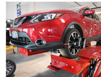
ADAS calibration cannot be performed until the wheels have been properly aligned and inspected for damage. Make any necessary alignment corrections before proceeding to ADAS corrections.
