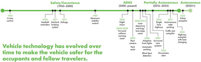
Anti-Lock Brakes (ABS) made it possible to create an Electronic Stability Control (ESC), which required The term Advanced Driver Assist System (ADAS) and ABS system, steering angle sensor and other sensors. is used to describe this technology The long-term goal is autonomous vehicles.
