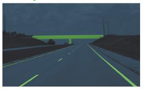
Imagine a vehicle equipped with emergency braking leaves the shop without a proper calibration and the camera is out of height adjustment (raised slightly horizontal) by even minimal degrees. The visual line of sight of the camera even slightly out of adjustment changes the responsiveness of the ADAS functions.
